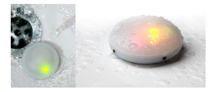
The Waterpebble has a smooth, pebble-like appearance and is designed to sit on the floor of a shower, recording the amount of time that water flows past it, thus measuring the amount of time a person spends in the shower. It aims to gradually reduce the time spent showering, by using a traffic light LED system to indicate when the user should finish.
